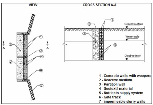
Figure 3: The construction scheme - solution 1.
