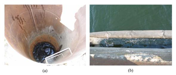
Figure 1: The pollution effects. (a) - Groundwater monitoring well;(b) - Surface water stream; actions aim to diminish the downstream pollution extending by using floating booms for collecting the oil products.
