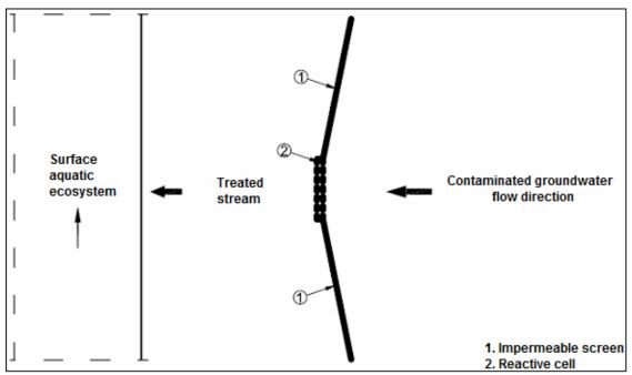
Figure 2: The principle scheme of the method.
