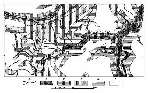
Figure 3 Simplified soil map of a part of the Eendrachtspolder near Rotterdam. After Edelman and unpublished survey of Scheepers. A) creek bed 1) calcareous sandy clay 2) calcareous clay 3) non-calcareous clay on a calcareous clay 4) deep non-calcareous clay 5) "katteklei"
