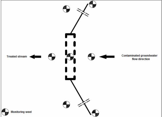
Figure 5: The positioning monitoring wells during the system's operation period scheme. **CONCLUSIONS**
