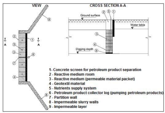
Figure 4: The construction scheme - solution 2.
